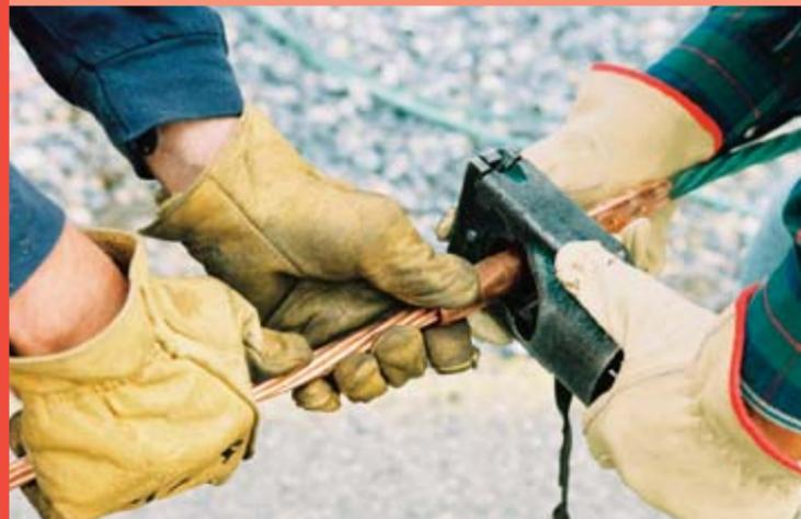
Personal Protective Equipment used in Cable Crimping
